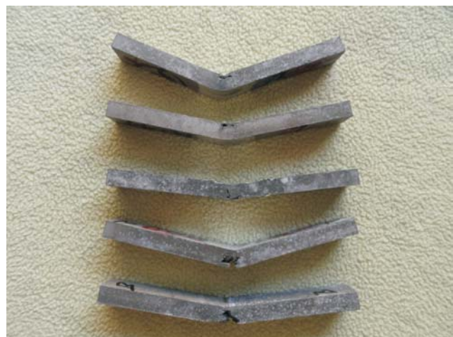
Fig. 5 (a) Typical bending specimens (b) Typical bend tested specimens after testing
