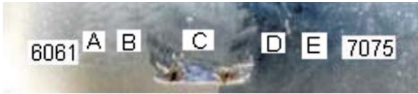
Fig. 4 The cross section of a FSW weld (900rpm, 90mm/min); 'A' denotes HAZ at AS; 'B' is the TMAZ at AS; 'C' is the SZ; 'D' is the TMAZ at RS; 'E' is the HAZ at RS; showing tunnel defect.
