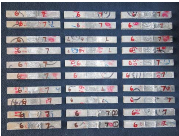
Fig. 5 (a) Typical bending specimens (b) Typical bend tested specimens after testing
