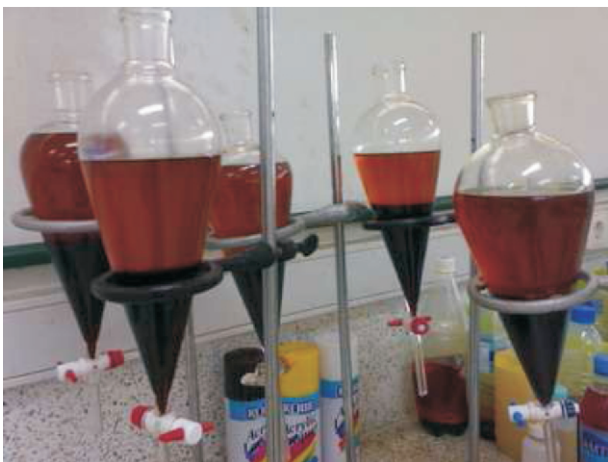
Fig. 9. Methyl ester and glycerin during the separation process
