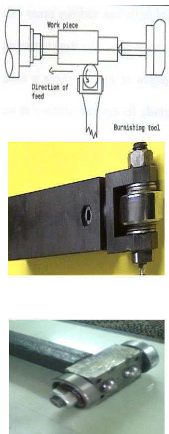
Figure 2 (a) Ball Burnishing tool (b) Roller burnishing tool (c) Combined burnishing tool
