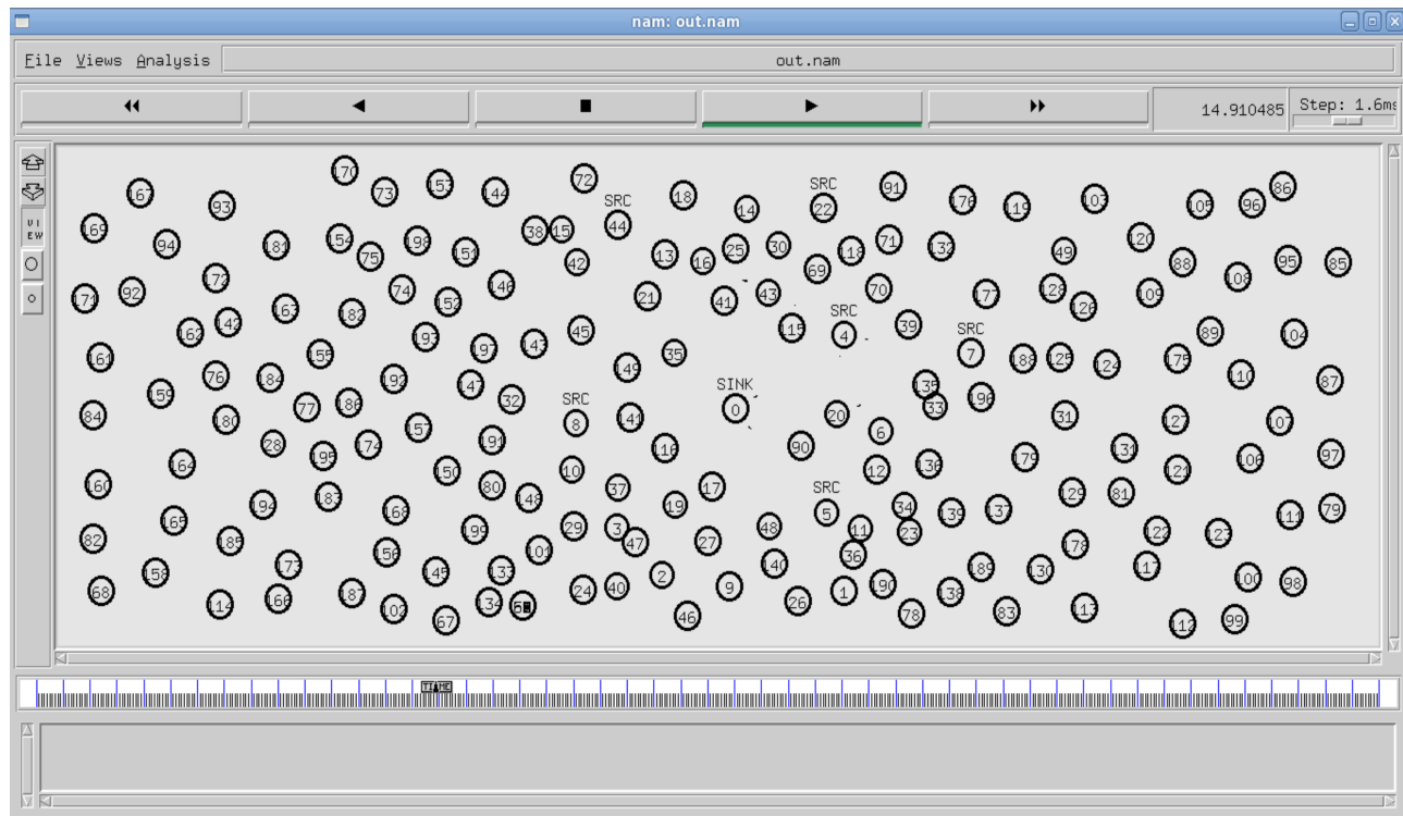
Fig. 3. Scenario with data transmission from 6 sources to 1 sink at 20kb data rate in network with 200 sensor nodes.
