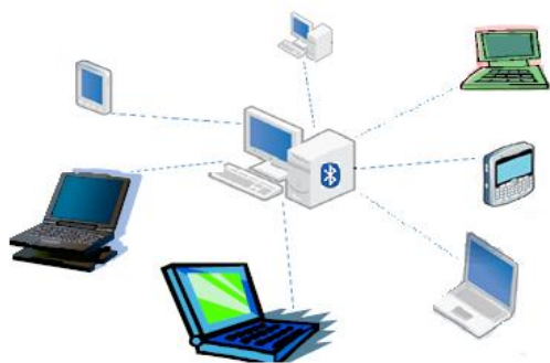
Fig.4 A Bluetooth with seven active node
