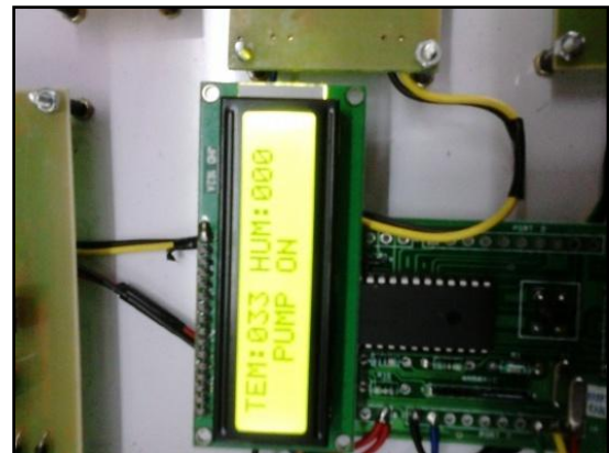
Fig. 4 Motor Pump is in on condition
