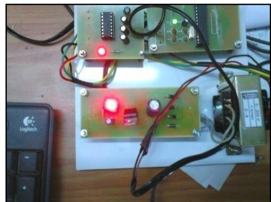
Fig.5 light blinking when the motor is in On condition
