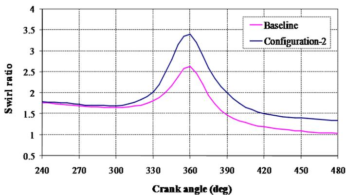
Fig.4 Average Swirl Ratio During Compression and Expansion
