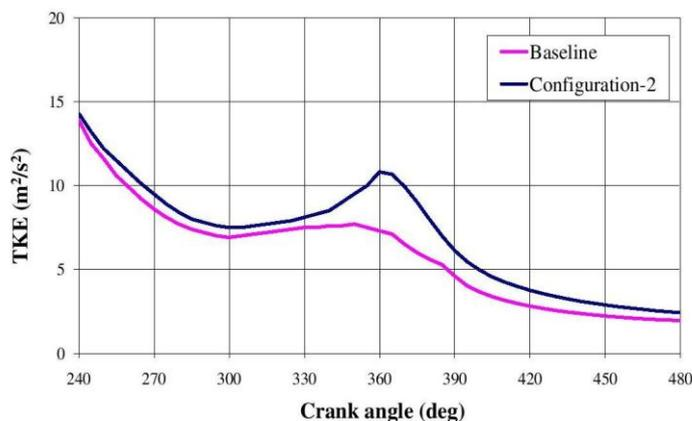
Fig.5 Average TKE Variation During Compression And Expansion
