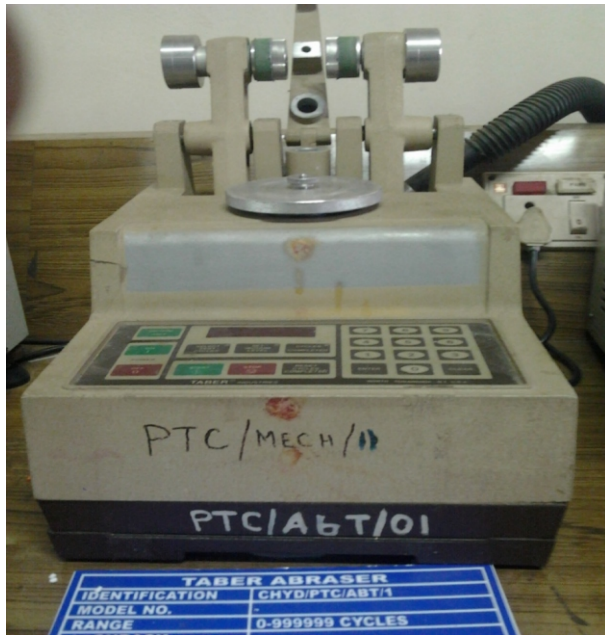
Fig. 2. Experimental setup for Wear Resistance test.
