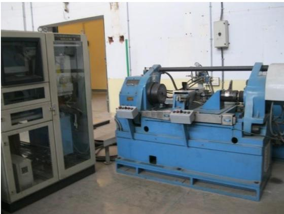
Fig. 1. Friction welding machine
