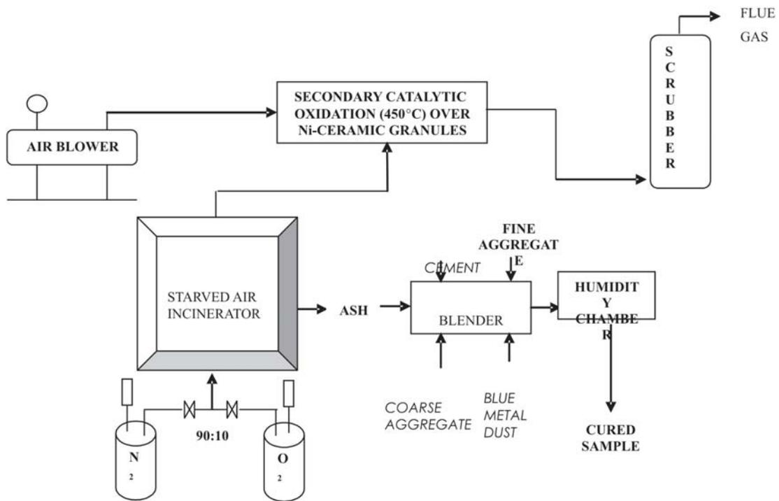
Fig. 1. Schematic Diagram of Starved Air Incineration Followed by S/S Process
