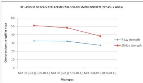
Fig 6. Behaviour of RCA % replacement in Geo-polymer concrete (fly ash + GGBS)
