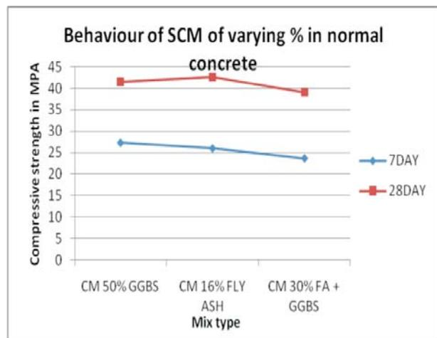
Fig 2. Behaviour of compressive strength verses different normal mixes of varying FA, GGBS
