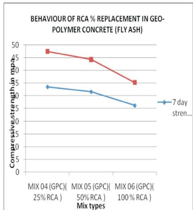
Fig. 5. Behavior of compressive strength verses different normal mixes RCA % replacement in Geo-polymer concrete (fly ash)
