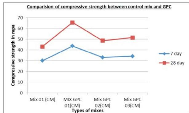
Fig 1. Behaviour of compressive strength verses different control mixes
