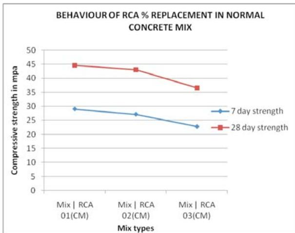
Fig 3. Behaviour of compressive strength verses different normal mixes RCA 25, 50,100% replacement in normal concrete mix
