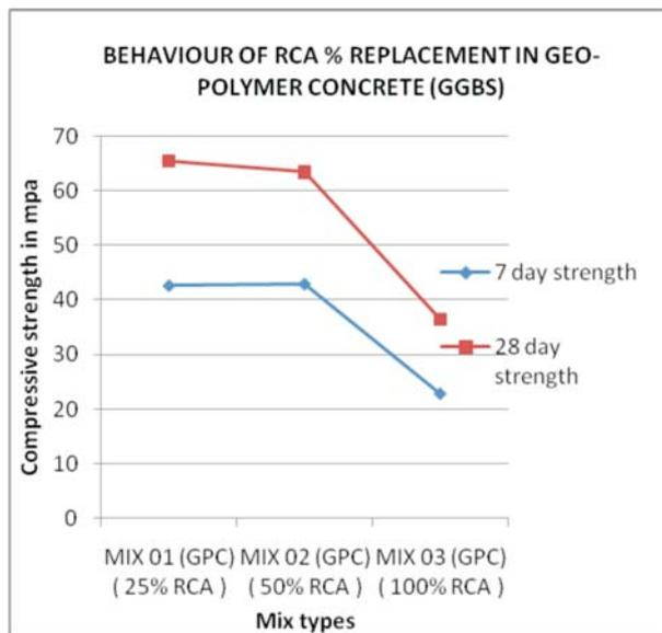
Fig 4. Behaviour of compressive strength verses different normal mixes RCA 25, 50,100% replacement in GPC mix
