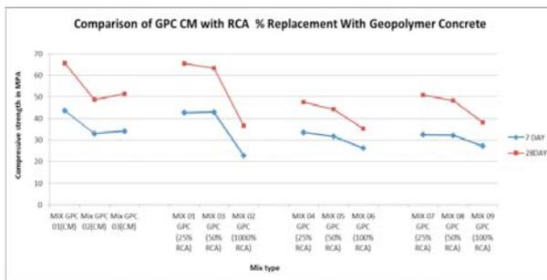
Fig 7. Graph of compressive strength of GPC (CM) with % RCA GPC mixes
