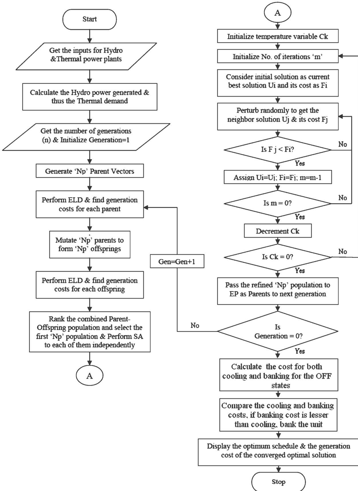
Fig. 1. EPSAM flowchart for Hydro-Thermal UCP
